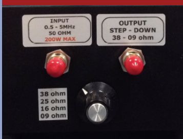
Impedance Matching Transformer
