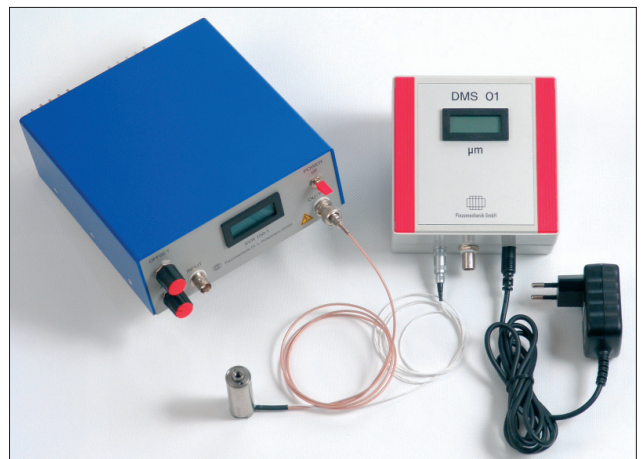
Fig. 6.4: Basic position control equipment. Piezo-actuator with strain gage position sensor. Position read out by DMS 01 unit. Piezo-actuator supply electronics SVR 150 (left)
