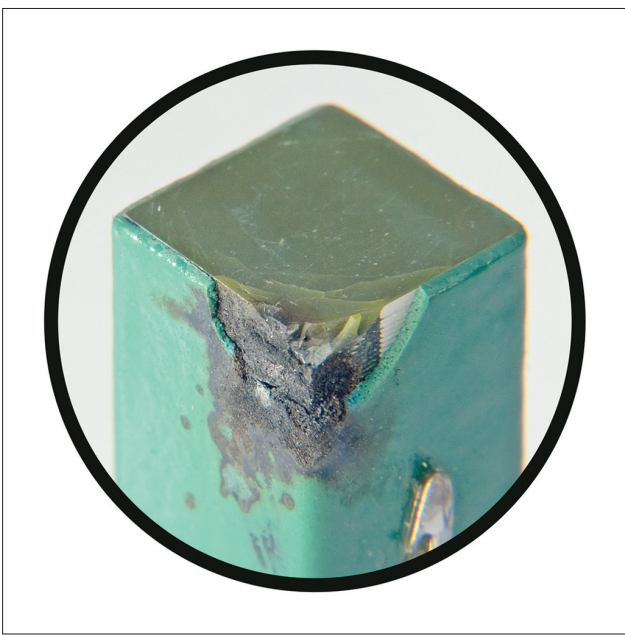
Fig. 7.1: Failed actuator stack, caused by a wrong coupling to the actuated mechanics. Local edge pressure exceeded ceramic's stability with subsequent electrical break down after approx. 800 hours.
